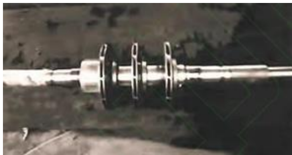
图 9 西安热工院采用的闭式叶轮压缩机 [48] Fig.9 The closed impeller compressor used in Xi'an Thermal Power Research Institute [48]
